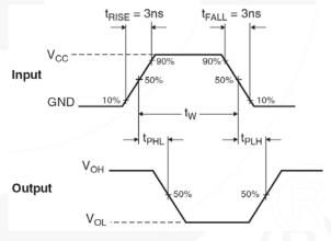
Figure 6. AC Waveforms
