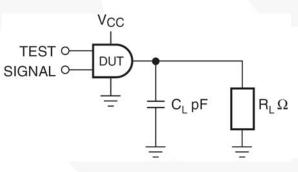
Figure 5. AC Test Circuit
