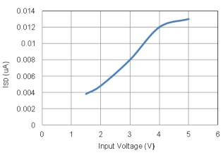
Operating Current vs Input Voltage (Differential output)
