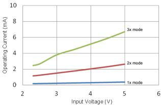
Operating Current vs Input Voltage (Single Ended Output)
