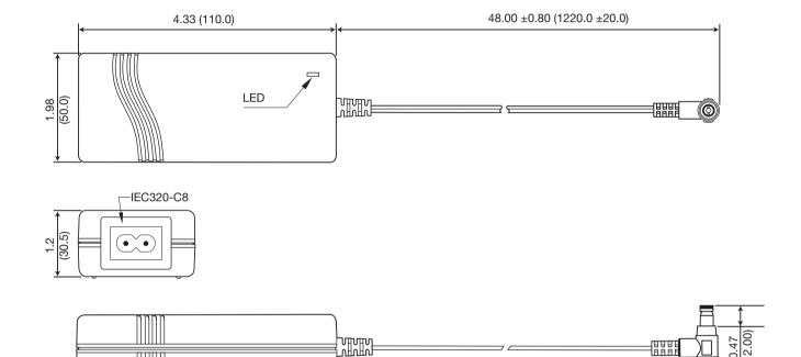
Output connector is right angle jack 0.22  $\times$  0.10  $\times$  0.47 (5.5  $\times$  2.5  $\times$  12.0), center postive. Weight: 0.49 lbs (220 g). Case tolerance:  $\pm$ 0.02 ( $\pm$ 0.5) All dimensions in inches (mm).
