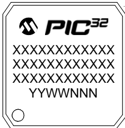
144-Lead TQFP (16x16x1 mm)
