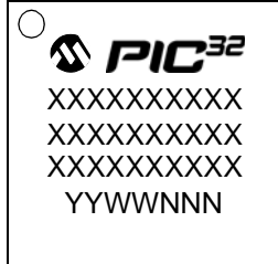
64-Lead QFN (9x9x0.9 mm)
