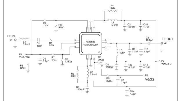
Figure 3. Schematic of Application Circuit Showing External Components
