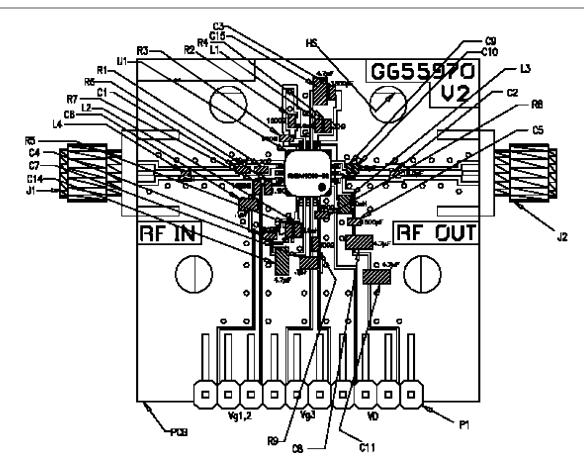
Figure 4. Layout of Test Evaluation Board (RMBA19500A-TB, G655971)
