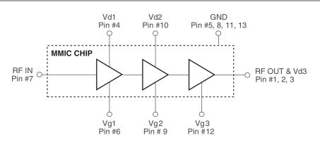
Figure 2. Functional Block Diagram
