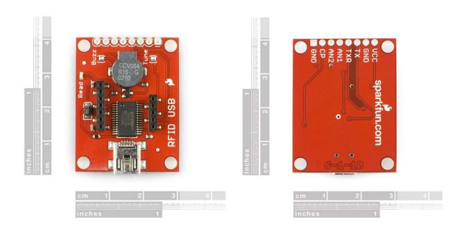
**Description:** The SparkFun RFID USB Reader is a simple to use, USB to serial base unit for the ID-3LA, ID-12LA, and ID-20LA readers. Simply plug a reader into the headers and attach a miniUSB cable. Open a terminal program of your choice at 9600bps 8N1, then scan your 125kHz ID tag and the unique 32-bit ID will be shown on the screen. The unit is based on a FTDI chip and comes with a read LED and buzzer.
