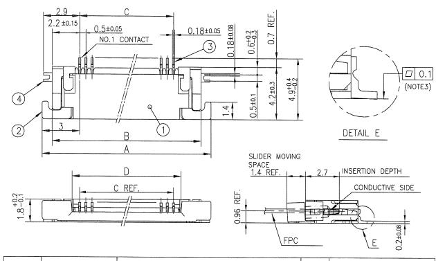
PARTS NAME PT. NO. MATERIAL Q'TY NOTE 13~35pin: LCP RESIN GLASS REINFORCED (UL94V-0) HOUSING 1 COLOR: BLACK (HALOGEN FREE) 4~12pin : POLYAMIDE RESIN GLASS REINFORCED (UL94V-0) PPS RESIN GLASS REINFORCED (UL94V-0) SLIDER COLOR: BLACK (HALOGEN FREE) 3 CONTACT n PLATING: GOLD PHOSPHOR BRONZE 4 MOUNTING PLATE PLATING: LEAD FREE
