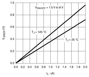
$V_{\mbox{\footnotesize DROP}}$  vs.  $I_{\mbox{\footnotesize L}}$  at  $V_{\mbox{\footnotesize IN}}$  = 4.5 V
