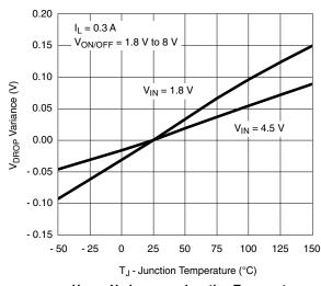
$\ensuremath{V_{DROP}}$  Variance vs. Junction Temperature
