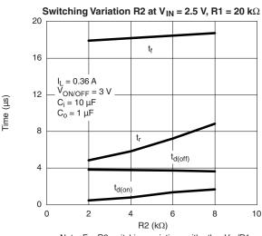
Note: For R2 switching variations with other V<sub>IN</sub>/R1 combinations See Typical Characteristics
