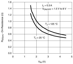
On-Resistance vs. Input Voltage
