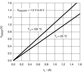
V<sub>DROP</sub> vs. I<sub>L</sub> at V<sub>IN</sub> = 1.8 V
