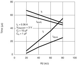
Switching Variation R2 at  $V_{IN} = 1.8 \text{ V}$ , R1 = 300 kW
