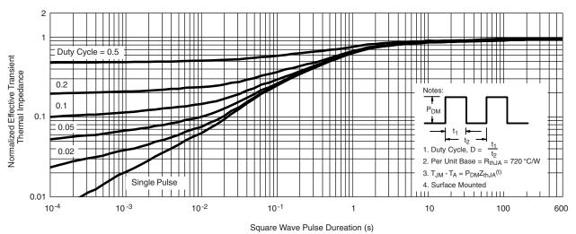
Normalized Thermal Transient Impedance, Junction-to-Ambient
