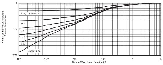
Normalized Thermal Transient Impedance, Junction-to-Foot
