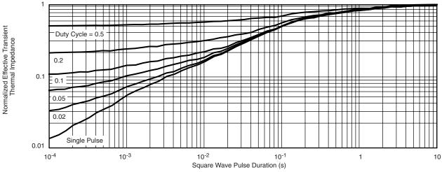
Normalized Thermal Transient Impedance, Junction-to-Foot
