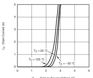
V<sub>GS</sub> - Gate-to-Source Voltage (V) **Transfer Characteristics**
