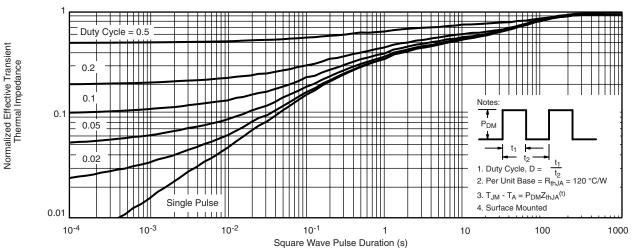
Normalized Thermal Transient Impedance, Junction-to-Ambient
