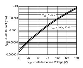
Gate Current vs. Gate-to-Source Voltage
