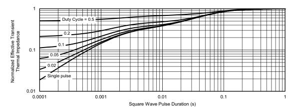
Normalized Thermal Transient Impedance, Junction-to-Case
