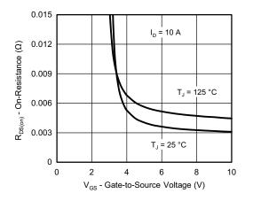
On-Resistance vs. Gate-to-Source Voltage
