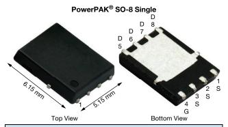
**PRODUCT SUMMARY**  $V_{DS} \overline{(V)}$ 30  $R_{DS(on)}$  max. ( $\Omega$ ) at  $V_{GS}$  = 10 V 0.0035  $R_{DS(on)}$  max. ( $\overline{\Omega}$ ) at  $V_{GS}$  = 4.5 V 0.0052 Qg typ. (nC) 11.2 60 a, g  $I_D(A)$ Configuration Single
