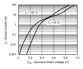
Source-Drain Diode Forward Voltage
