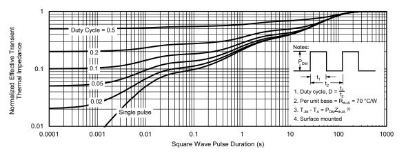
Normalized Thermal Transient Impedance, Junction-to-Ambient
