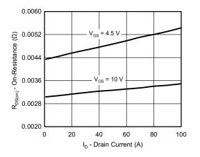
**On-Resistance vs. Drain Current and Gate Voltage**
