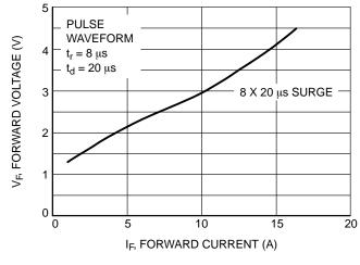
Figure 5. 8 x 20 μs V<sub>F</sub>
