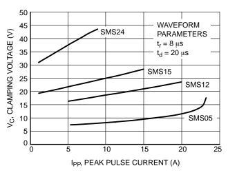
Figure 4. Clamping Voltage versus
