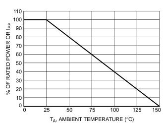
Figure 2. Power Derating Curve
