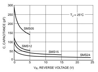
Figure 6. Typical Capacitance (SMS05 Series)
