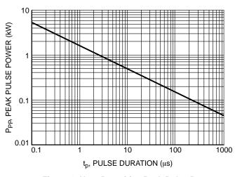
Figure 1. Non-Repetitive Peak Pulse Power versus Pulse Time
