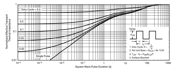
Normalized Thermal Transient Impedance, Junction-to-Ambient
