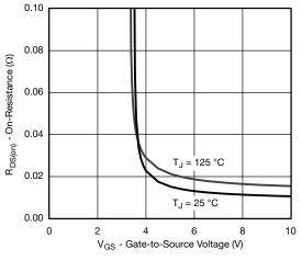
On-Resistance vs. Gate-to-Source Voltage
