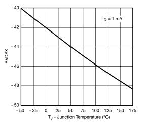
Breakdown Voltage vs. Junction Temperature
