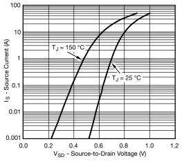
Source Drain Diode Forward Voltage
