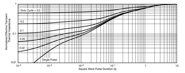
Normalized Thermal Transient Impedance, Junction-to-Foot
