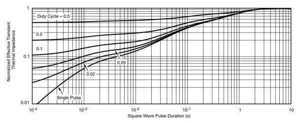
Normalized Thermal Transient Impedance, Junction-to-Case
