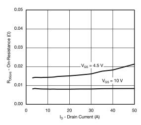
On-Resistance vs. Drain Current
