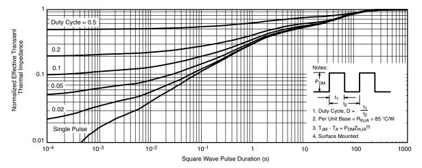
Normalized Thermal Transient Impedance, Junction-to-Ambient
