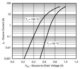
**Source Drain Diode Forward Voltage**
