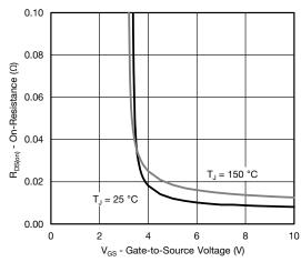
On-Resistance vs. Gate-to-Source Voltage
