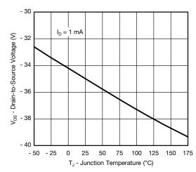
Drain Source Breakdown vs. Junction Temperature
