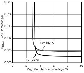
**On-Resistance vs. Gate-to-Source Voltage**
