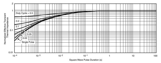
Normalized Thermal Transient Impedance, Junction-to-Case
