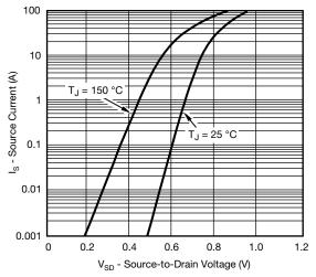
Source Drain Diode Forward Voltage
