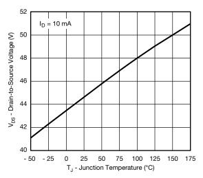
Drain Source Breakdown vs. Junction Temperature
