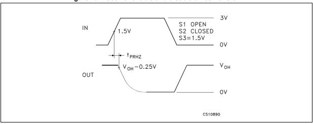
Figure 20. Receiver enable and disable times waveform
