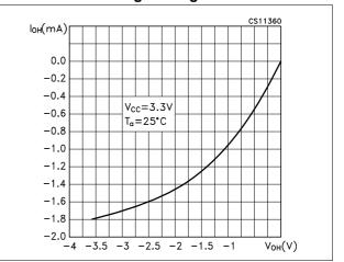
Figure 23. Low level driver output capability
