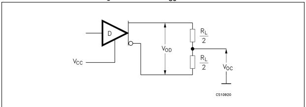
Figure 4. Driver  $V_{\mbox{\scriptsize OD}}$  with varying common mode voltage test load
