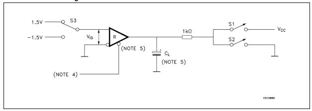
Figure 17. Receiver enable and disable times waveform 3٧ S1 OPEN IN 1.5٧ S2 CLOSED S3=1.5V  $t_{\mathsf{PRZH}}$ †<sub>PRSH</sub>  $V_{OH}$ OUT ٥٧ CS10870
