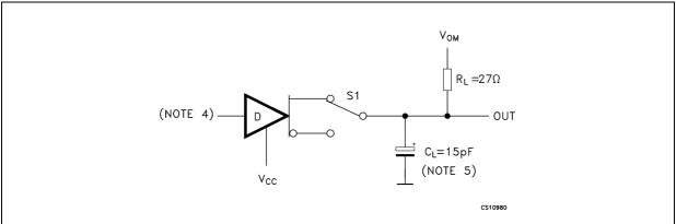
Figure 11. Drive propagation time waveform
