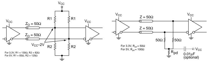
Figure 3a. Parallel Thevenin-Equivalent Termination
