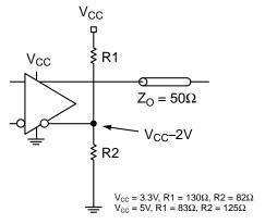
Figure 3c. Terminating Unused I/O
