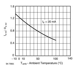
Fig. 8 - Relative Radiant Intensity/Power vs. Ambient Temperature
