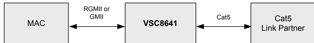
Figure 3. RGMI or GMI to Cat5 Block Diagram
