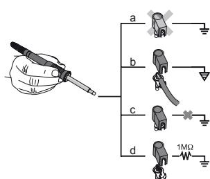
Four variants are possible by connecting the 3.5 mm jack socket differently:
