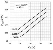
Fig. 6:  $V_{\text{SET}}$  versus Input Voltage at  $I_{\text{LED}} = 330 \text{mA}$
