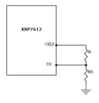
Fig. 21: V<sub>TH</sub> Voltage
