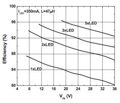
Fig. 5: Efficiency versus Input Voltage
