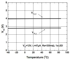
Fig. 11: Thermal Regulation Threshold versus Temperature
