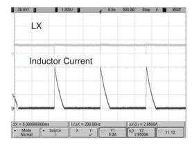
Fig. 15: Short Circuit  $V_{IN}$ =12V
