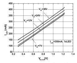
Fig. 9: LED Current versus EN/DIM Voltage
