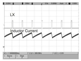
Fig. 12: Switch Waveform  $V_{\text{IN}}$ =12V,  $I_{\text{LED}}$ =350mA, 3 LEDs
