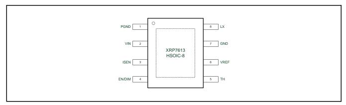
Fig. 3: XRP7613 Pin Assignment
