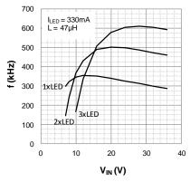
Fig. 16: frequency versus input voltage,  $I_{LED}$ =330mA
