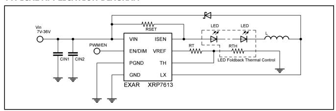
Fig. 1: XRP7613 Application Diagrams
