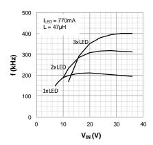
Fig. 17: frequency versus input voltage,  $I_{LED}$ =770mA
