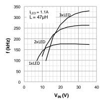
Fig. 18: frequency versus input voltage,  $I_{\text{LED}}=1.1A$
