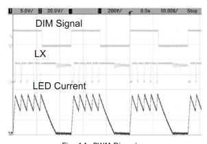
Fig. 14: PWM Dimming  $V_{\text{IN}}$ =24V, Duty Cycle = 50%,  $f_{\text{PWM}}$ =40kHz
