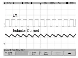
Fig. 13: Switch Waveform  $V_{IN}=12V$ ,  $I_{LED}=700$ mA, 1 LED
