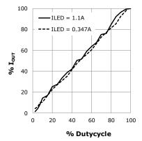
Fig. 19: PWM dimming at 25kHz,  $V_{\text{IN}}$ =24V, 3xLED, L=47 $\mu$ H
