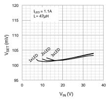
Fig. 8:  $V_{\text{SET}}$  versus Input Voltage at  $I_{\text{LED}}$ =1.1A
