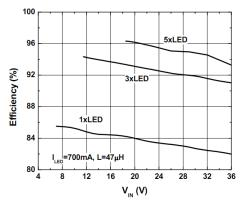
Fig. 4: Efficiency versus Input Voltage
