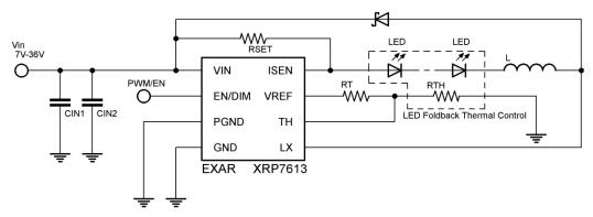
Fig. 22: Typical Application Diagram
